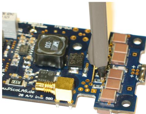
If you want to measure high-frequency floating signals we strongly recommend to use high-quality differential probes e.g. Tektronix P7240. Beware: Some of them have an operating limit of only few volts. Don't destroy them! The voltage across the output connectors is too high for most ultrafast probes!
