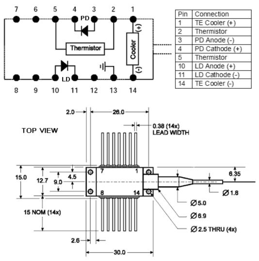
The driver is connecting pin 9 & 10 and pin 11 & 12 together. Pitch of the legs: 2.5 mm.
